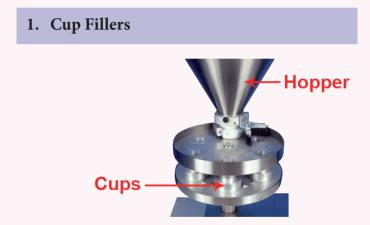
The material is filled in the top hopper from where it falls below in a circular cup whose height can be adjusted to adjust the volume. The volume of the cup is calibrated to the weight of the material to be packed. As the disc rotates the cups fill below the hopper and when they reach the discharge point the material is discharged in the pouch.
