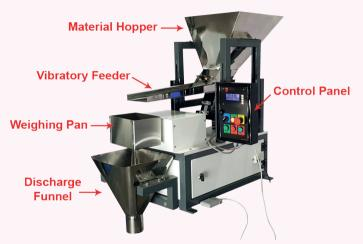
These filling systems actually fill the material by weight. The material flows through the hopper to the vibratory feeder tray which has two modes: coarse mode and fine mode for trickle feed and higher accuracy. From here it falls in the weighing pan which is mounted on a load cell where it is accurately weighed before the material is finally discharged into the bagging system.
