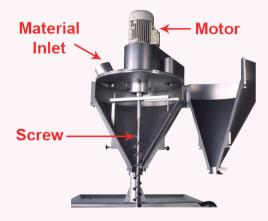
The material that is loaded in the hopper is dosed down into the pouch using a screw. The rotation of the screw pushes the material down in the pouch. Accurate control of the screw rotation is important for accurate dispensation. The material discharged in one rotation depends on the pitch of the screw. Nevertheless, this is also a volumetric system as material that can be filled in one pitch of the screw is dispensed in one rotation.
